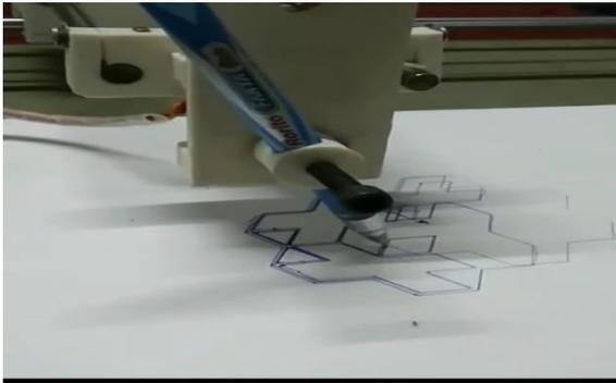
the command to run the device. The program will be transferred via Arduino and then loaded into the plotter machine to start machining. After completing its zero position settings and testing, the plotter machine was fully functional ready to work.
