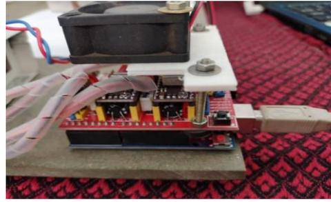
4. **3d printed bracket:** In this mahine some 3d printed bracket are used for mounting or support stepper motor . it is a plastic material and lighter in weight .
